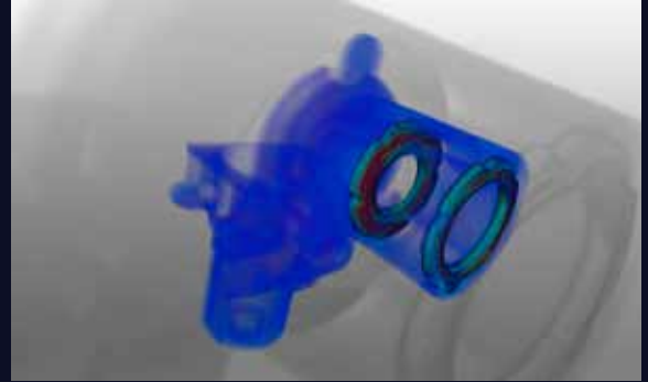
Casting Inspection Image : North Star Imaging
