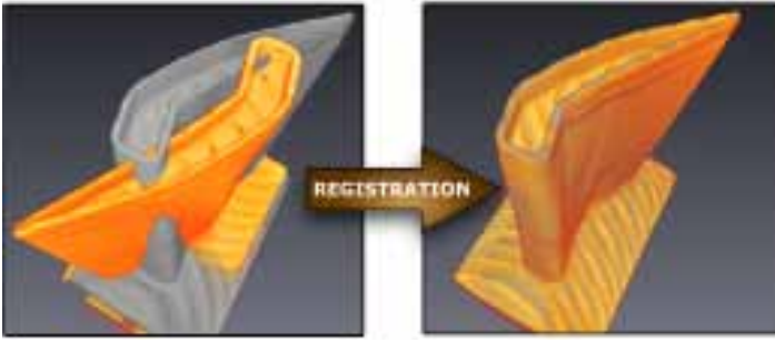
Advanced image registration: fusion of multi-modal data (Scan, CAD model, etc.) to perform variance comparison
